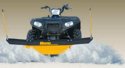
The dual flared wing moldboard design, coupled with the 65° attack angle, provides scoop and funnel discharge action.
