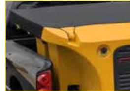
**Built-in tarp hooks** are engineered into the hopper making tarp installation and removal quicker and easier. Tarp comes standard on DLX model.
