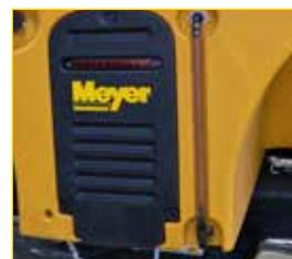
**Rear cover** protects auger motor from salt and debris.
