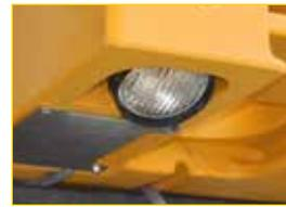
**Integrated work light** illuminates spread area and helps in maintenance operations. LED light standard on DLX model, halogen light on standard model.
