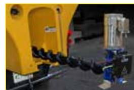
**Auger assembly** can easily be removed for maintenance or inspection.
